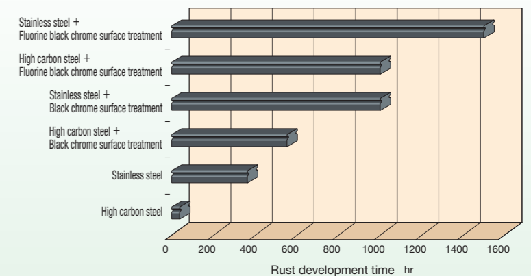
Corrosion resistance comparison based on humidity cabinet test*
