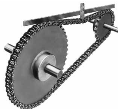
Determining chain sag
