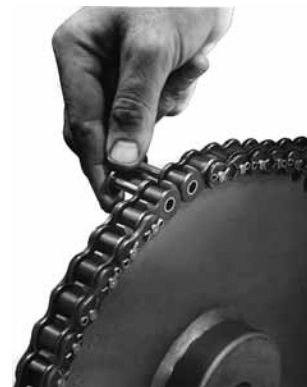
Inserting connecting link
