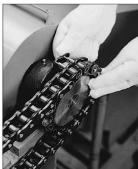
Fig. 8 Connecting on a sprocket
