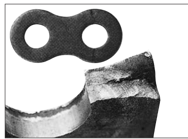
② Fatigue fracture By repeatedly applying a load past its fatigue limit (fatigue strength), the fatigue will start at holes and then cause sudden chain breakage.
