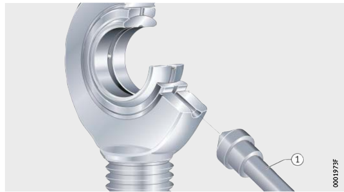
Figure 5 Relubrication via hole
